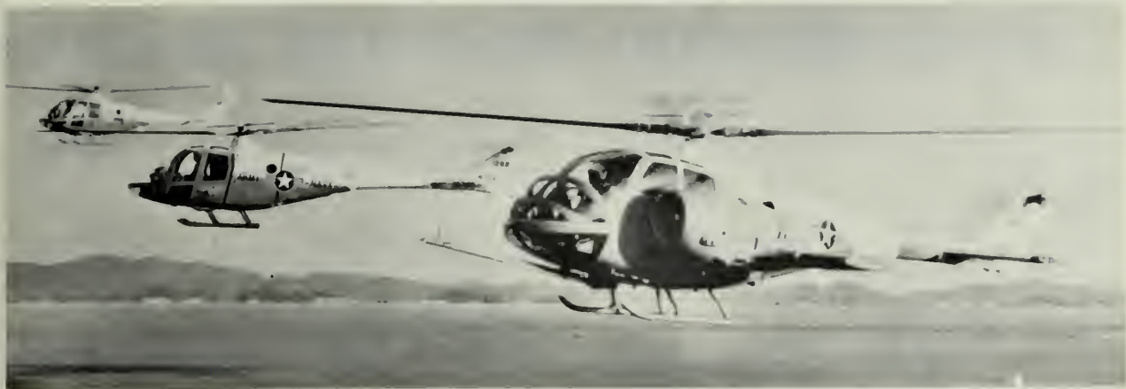
FAMILY PORTRAIT of new XH-51 helicopters shows XH-51N (top), built for NASA; HX-51A, built under a joint Army-Navy program (center); and winged version of XH-51A, which is fastest known rotorcraft, with speed of 242 mph.
